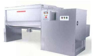
The Ribbon Blender does homogenous mixing of powder and granules of different densities. The Blender consists of a Semi-cylindrical shell inside which rotates a shaft welded with spiral inner and outer ribbons.
